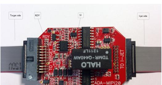
The adapter is automatically recognized by the C-SPY, and the adapter powers up and the green RDY LED is turned on.
