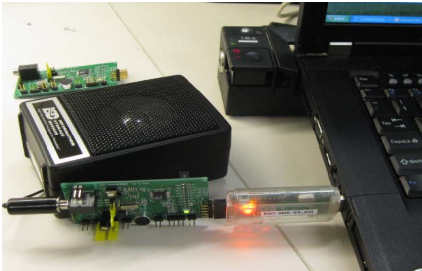
Figure 5 – A complete evaluation environment for ISD15100 device
