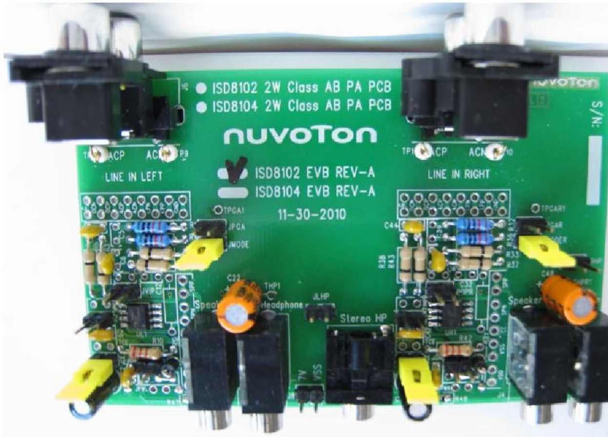
Figure 2: ISD-DEMO8102 EVB Jumpers Setting
