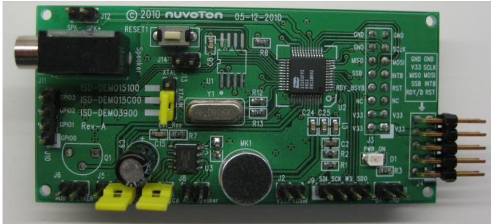
Figure 1 – Top view of ISD-DEMO15100/15C00/3900 Rev-A board
