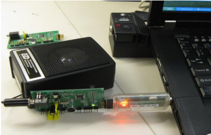
Figure 5 – A complete evaluation environment for ISD15100 device
