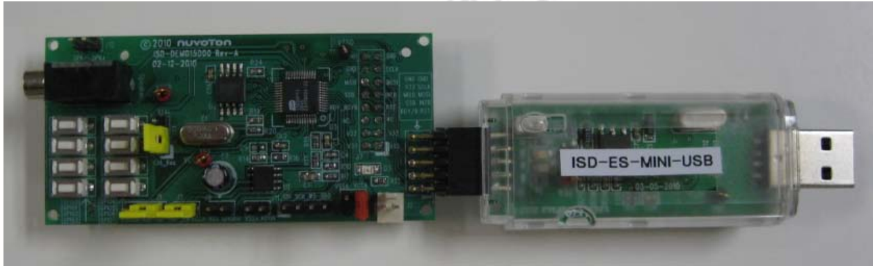
Figure 3 – ISD_DEMO15D00 connected with ISD-ES_MINI_USB (dongle) board
