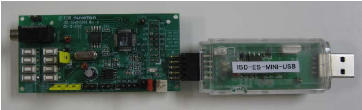
Figure 3 – ISD_DEMO15D00 connected with ISD-ES_MINI_USB (dongle) board
