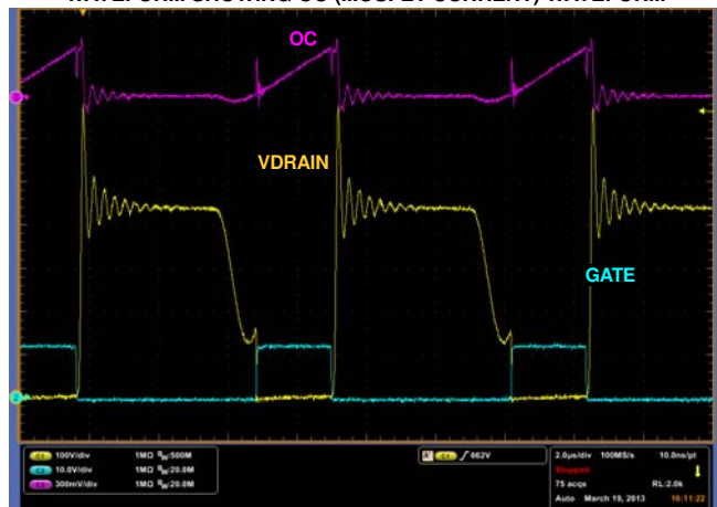
FIGURE 21. TRACE 1 - DRAIN VOLTAGE [100V/DIV]; TRACE 2 - GATE [10V/DIV]; TRACE 3 - DRAIN CURRENT OR OC [300mV/DIV]
