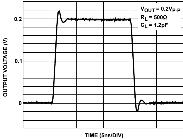
FIGURE 14. SMALL SIGNAL TRANSIENT RESPONSE; R_L = 500\Omega
