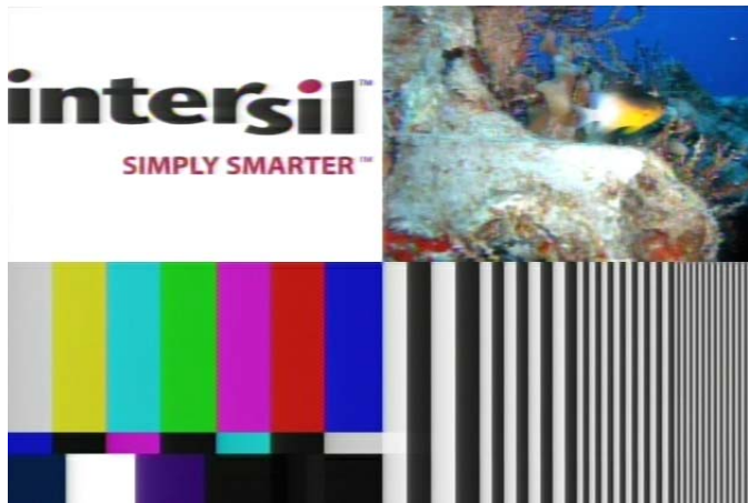
FIGURE 25. TEST PATTERN IMAGE AFTER 2000 FEET OF UNCOMPENSATED RG-59 COAX
