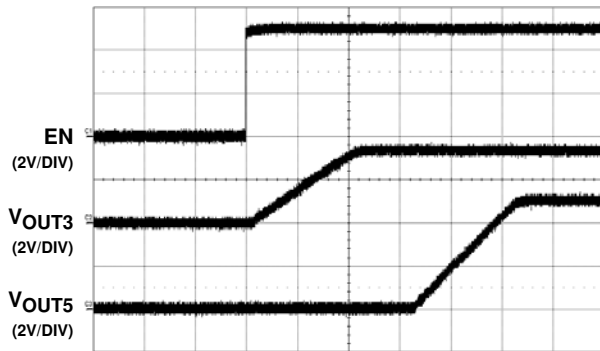
FIGURE 23. DELAYED START WAVEFORMS (EN5 = REF)
