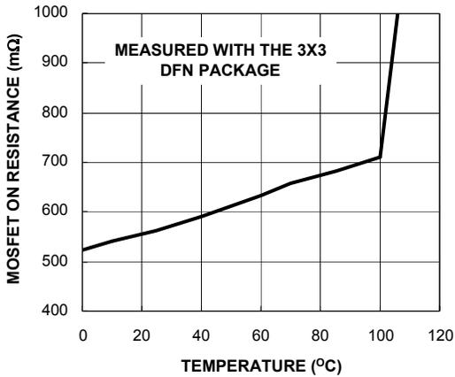
FIGURE 9.  $r_{DS(ON)}$  vs TEMPERATURE AT 3.7V OUTPUT
