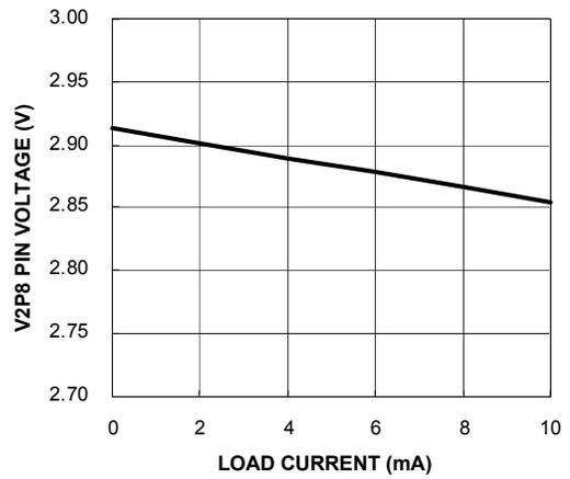
FIGURE 8. V2P8 OUTPUT vs ITS LOAD CURRENT
