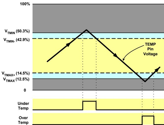
FIGURE 25. CRITICAL VOLTAGE LEVELS FOR TEMP PIN
