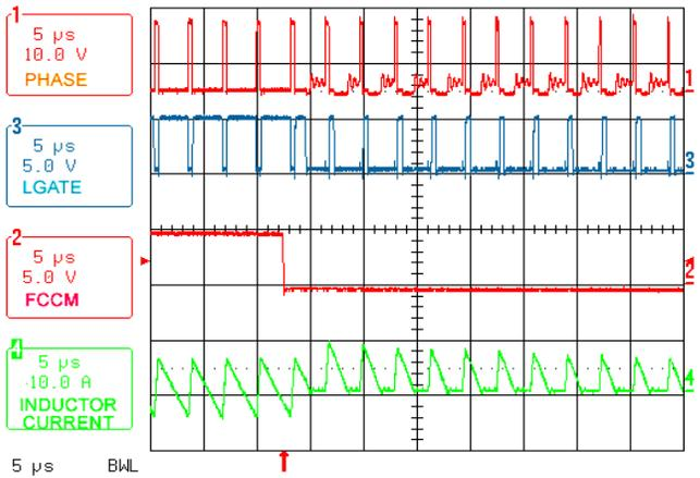
FIGURE 5. CCM TO DCM TRANSITION AT NO LOAD
