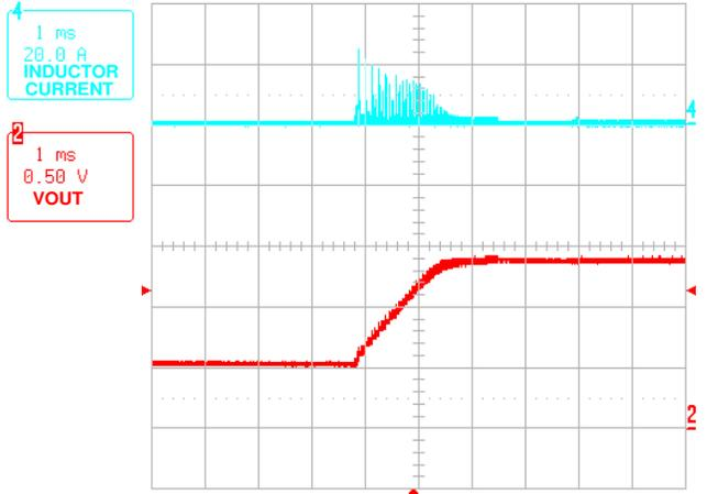
FIGURE 7. PRE-BIASED STARTUP IN DCM MODE (FCCM = LO)
