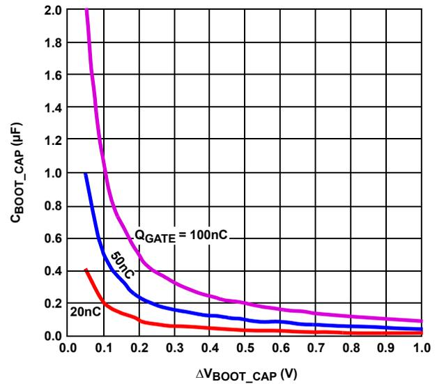
FIGURE 8. BOOTSTRAP CAPACITANCE vs BOOT RIPPLE VOLTAGE
