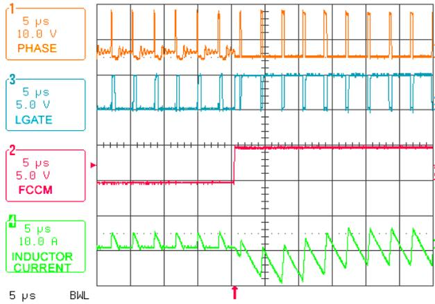
FIGURE 4. DCM TO CCM TRANSITION AT NO LOAD
