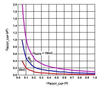
FIGURE 8. BOOTSTRAP CAPACITANCE vs BOOT RIPPLE VOLTAGE
