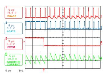
FIGURE 5. CCM TO DCM TRANSITION AT NO LOAD
