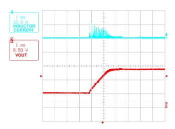
FIGURE 7. PRE-BIASED STARTUP IN DCM MODE (FCCM = LO)
