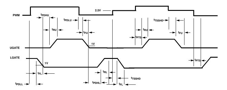
FIGURE 1. TIMING DIAGRAM
