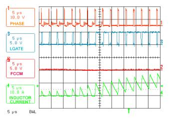
FIGURE 2. LOAD TRANSIENT (0 to 30A, 3-PHASE)
