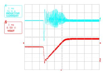
FIGURE 6. PRE-BIASED STARTUP IN CCM MODE (FCCM = HI)
