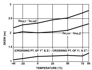
FIGURE 13. DRIVER SKEW vs TEMPERATURE (ISL8485, ISL8490, ISL8491)
