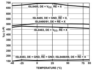
FIGURE 9. SUPPLY CURRENT vs TEMPERATURE
