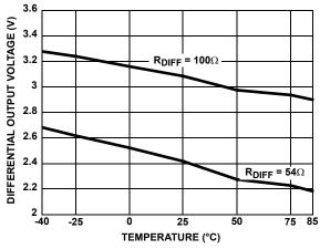
FIGURE 7. DRIVER DIFFERENTIAL OUTPUT VOLTAGE vs TEMPERATURE
