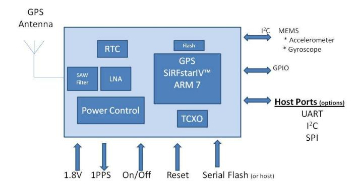
Figure 1 Inventek's ISM420R1-CX General Block Diagram
