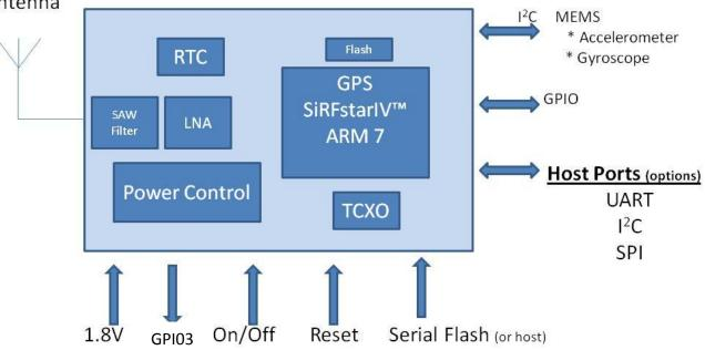
Figure 1 Inventek's ISM480F1 General Block Diagram
