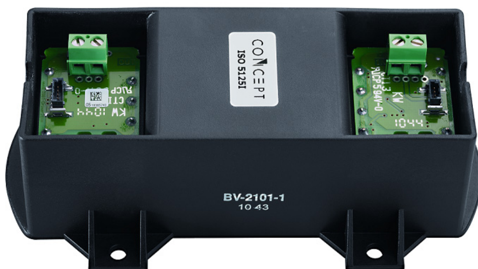
Fig. 1 Power Supply ISO5125I
