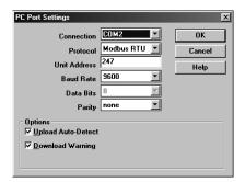
The Communications Settings window allows you to set up the software properly to perform a download.
