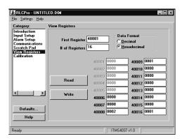
The View Registers category can be used as a method of diagnostics. Use the ITMS Register Table as a reference of register assignments and data.
