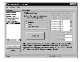
The ITMS is fully calibrated from the factory. Recalibration is recommended every two years. Each range has its own internal references that are recalled when the range is selected. This allows independent calibration for each range. All calibration settings are stored in the E<sup>2</sup>PROM. Calibration may be performed by using SFIMS software or MODBUS commands.
