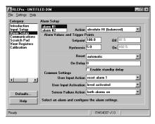
Action: Alarm 1 can be programmed for 5 modes of operation, Alarm 2 has 9 possible modes. See Setpoint Alarm figures for illustration.
