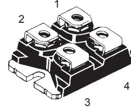
1 = Source      3 = Drain / Diode anode
