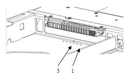
The key is a pin positioned in one of six holes on the bottom of the shelf
