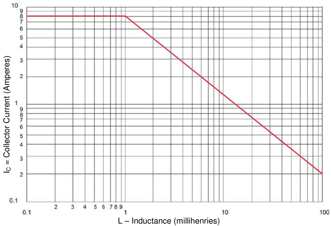
FIGURE 2 Safe Operating Area for switching between saturation and cutoff (unclamped inductive load)
