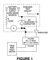
Noise Density Measurement Circuit
