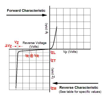
**FIGURE 4**Zener Diode Characteristics and Symbol Identification
