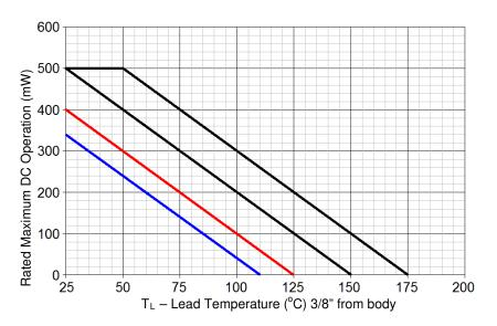
FIGURE 2 – Temperature-Power Derating Curve
