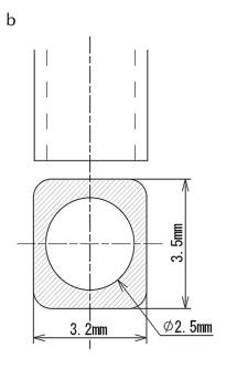
\* Nozzle with chamfering is recommended
