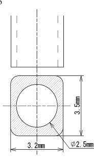
\*Nozzle with chamfering is recommended
