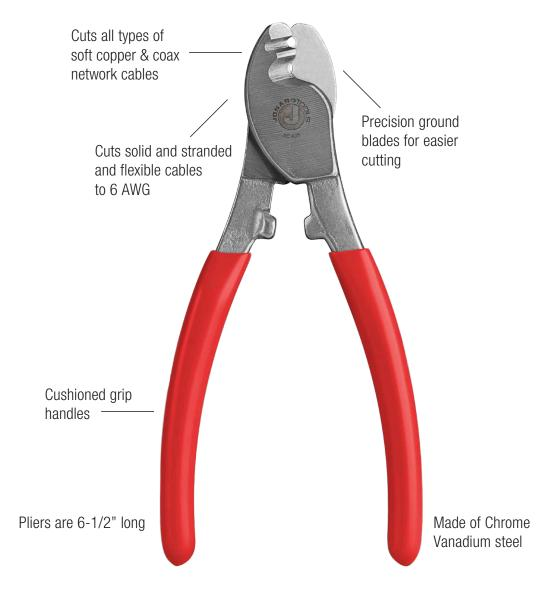
**IMPORTANT:** Not for use on steel, aluminum alloy or hard drawn copper cables
