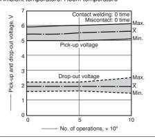
7-(2). Electrical life test (Motor free) Sample: JJM1-12V, 6pcs. Load: Inrush 25A, Steady 5A, Brake current 18A 14V DC, Power window motor load (Free condition). Operating frequency: ON 0.5s, OFF 9.5s
