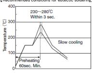
[Recommended condition for Pb-free soldering]
