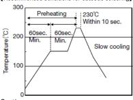
[Recommended condition for Pb-free soldering]
