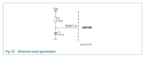
The external resistor and capacitor provide a simple reset operation when connected to the RESET\_N pin but are not necessary.
