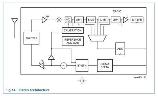
The radio comprises a low-IF receive path and a direct modulation transmit path, which converge at the TX/RX switch. The switch connects to the external single-ended matching network, which consists of two inductors and a capacitor. This arrangement creates a 50  $\Omega$  port and removes the need for a balun. A 50  $\Omega$  single-ended antenna can be connected directly to this port.
