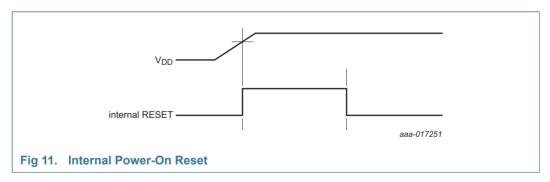
When the supply drops below the POR 'falling' threshold, it will retrigger the reset. On platform with higher power (e.g. light bulb, smart plug) it is recommended to use this external circuit to avoid unexpected reset due to spurs.
