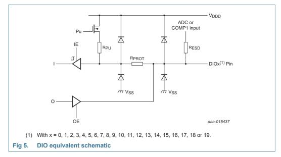
In reset, the digital peripherals are all off and the DIO pins are set as high-impedance inputs. During sleep and deep sleep, the DIO pins retain both their input/output state and the output level that was set at the start of sleep. If the DIO pins were enabled as inputs and the interrupts were enabled, then these pins may be used to wake up the JN5169 from sleep.
