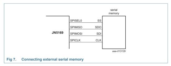
The contents of the external serial memory may be encrypted. The AES security processor combined with a user programmable 128-bit encryption key is used to encrypt the contents of the external memory. The encryption key is stored in the Flash memory
