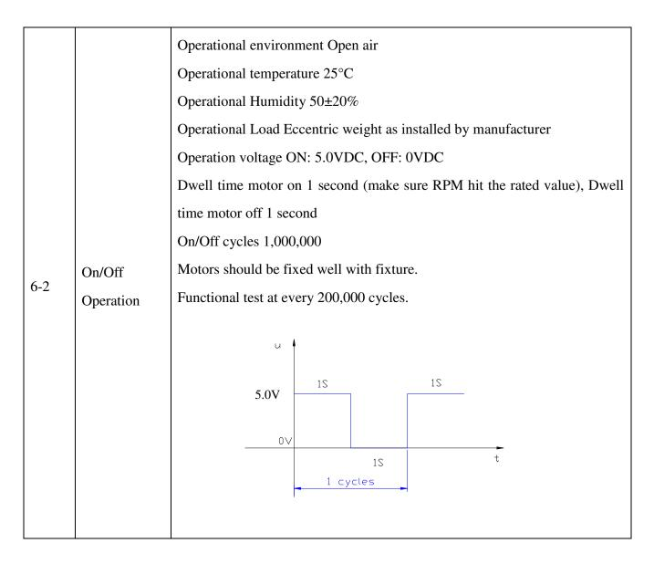
Before/After life test, measuring the rated load specification. Motor life is judged to come to an end. When
