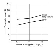
1-(2). Coil temperature rise (15A) Measured portion: Inside the coil Contact carrying current, 15A Ambient temperature: Room temperature, 85°C 185°F
