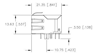
DIMENSIONS ARE IN MILLIMETERS [INCHES] WITH THE FOLLOWING TOLERANCES: [INCHES] ARE FOR REFERENCE ONLY.  $X.XX = \pm 0.25$  [ $\pm .010$ ]
