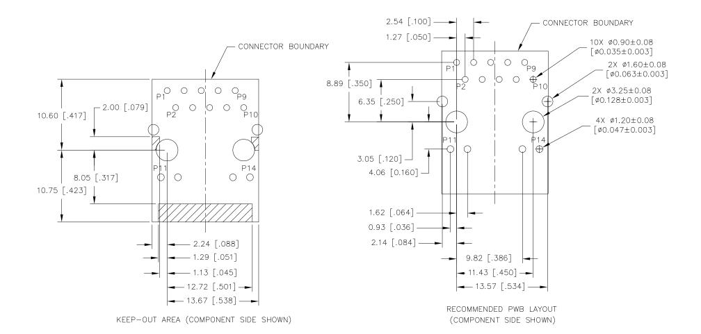
DIMENSIONS ARE IN MILLIMETERS [INCHES] WITH THE FOLLOWING TOLERANCES: [INCHES] ARE FOR REFERENCE ONLY.  $X.XX = \pm 0.10$  [ $\pm .004$ ]
