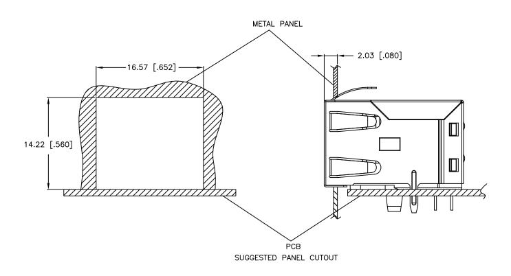
DIMENSIONS ARE IN MILLIMETERS [INCHES] WITH THE FOLLOWING TOLERANCES: [INCHES] ARE FOR REFERENCE ONLY.  $X.XX = \pm 0.10 \ [\pm .004]$
