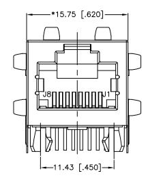
DIMENSIONS ARE IN MILLIMETERS [INCHES] WITH THE FOLLOWING TOLERANCES: [INCHES] ARE FOR REFERENCE ONLY.  $X.XX = \pm 0.25$  [ $\pm .010$ ]
