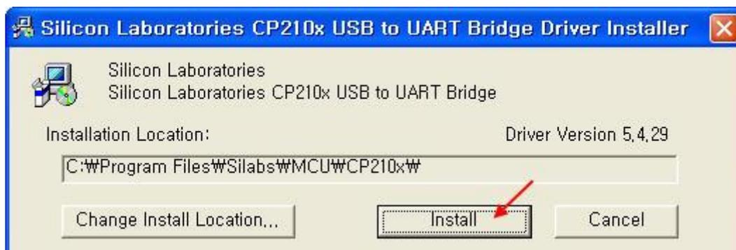
(D) If the driver is not installed, it can be installed manually when CP210x is connected to the PC. The driver is located in “C:\Program Files\Silabs\MCU\CP210x” folder.
