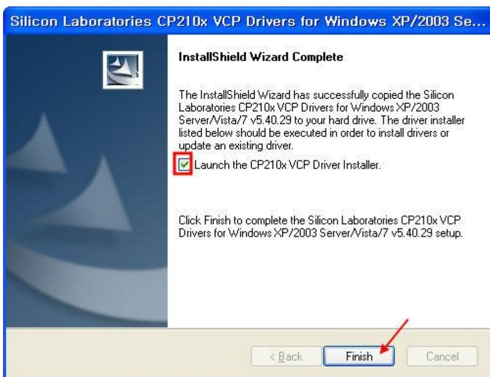
If it is not checked, it can be reinstalled later by executing “C:\SiLabs\MCU\CP210x\Windows...Vista\_7\CP210xVCPInstaller.exe”.
