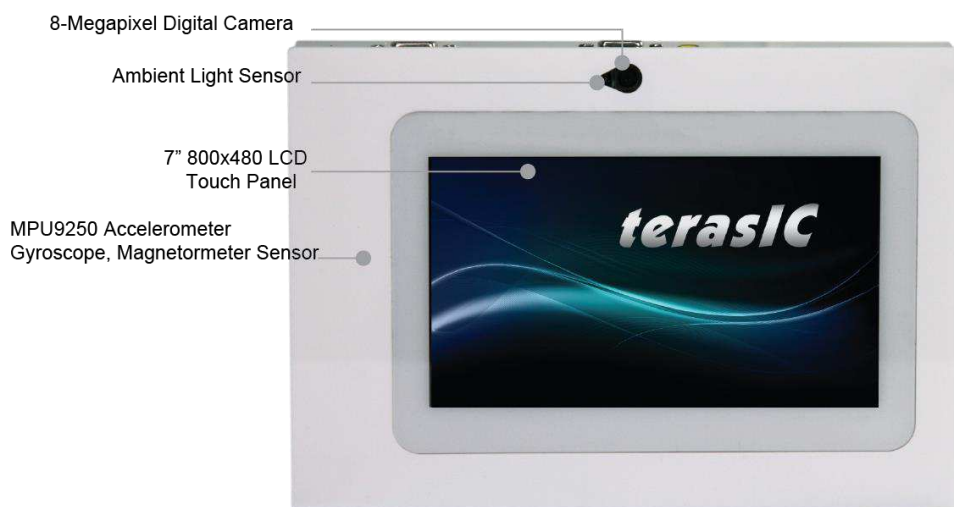
Figure 2-1 VEEK-MT2-C5SOC PCB and Component Diagram (top view)
