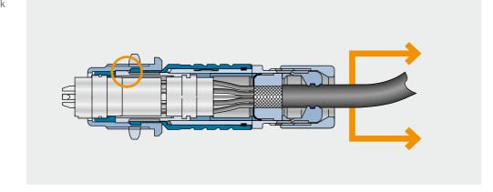
But pulling on the outer housing will cause the fingers to emerge from the locking groove, making it easy to disconnect the connector.
