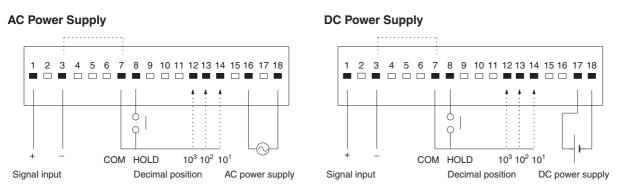
Note: 1. Terminals 3 and 7 of the AC and DC models are not internally insulated. Connect a relay with high contact reliability and insulation (with a minimum load current of 0.3 mA) or a photocoupler with high insulation (with a residual voltage of 1 V max. and a current leakage of 0.1 mA max.) to these terminals for external control.
