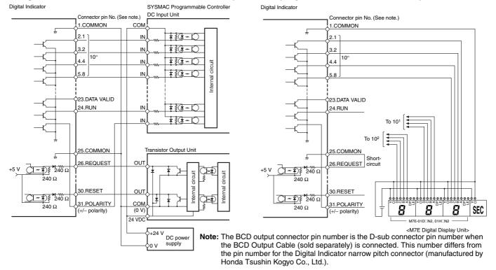
Refer to the following User's Manual for application precautions and other information required when using the Digital Indicator: K3HB-R/P/C Digital Indicator User's Manual (Cat. No. N136) The manual can be downloaded from the following site in PDF format: OMRON Industrial Web http://www.fa.omron.co.jp
