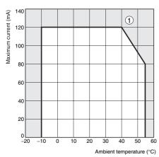
Note: 1. The above values were obtained under test conditions with the standard mounting. The derating curve will vary with the mounting conditions, so be sure to adjust accordingly.
