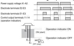
When the liquid level reaches E1 (indicator turns ON), the pump starts.
