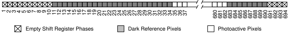
Figure 13. Line Timing Diagram – Single Register Output
