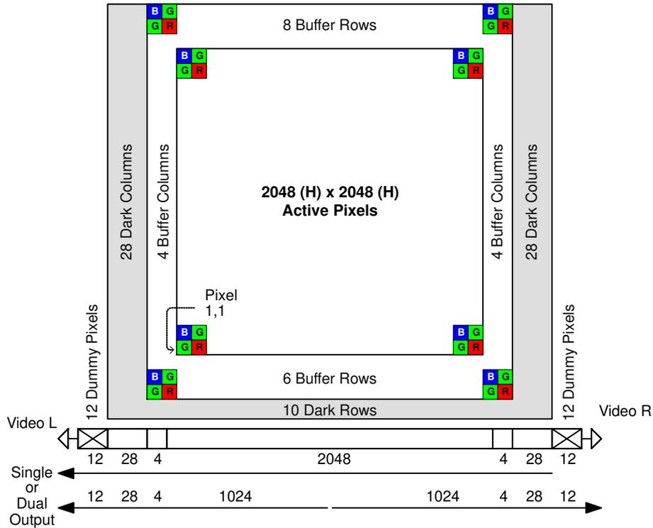
Figure 2. Sensor Architecture
