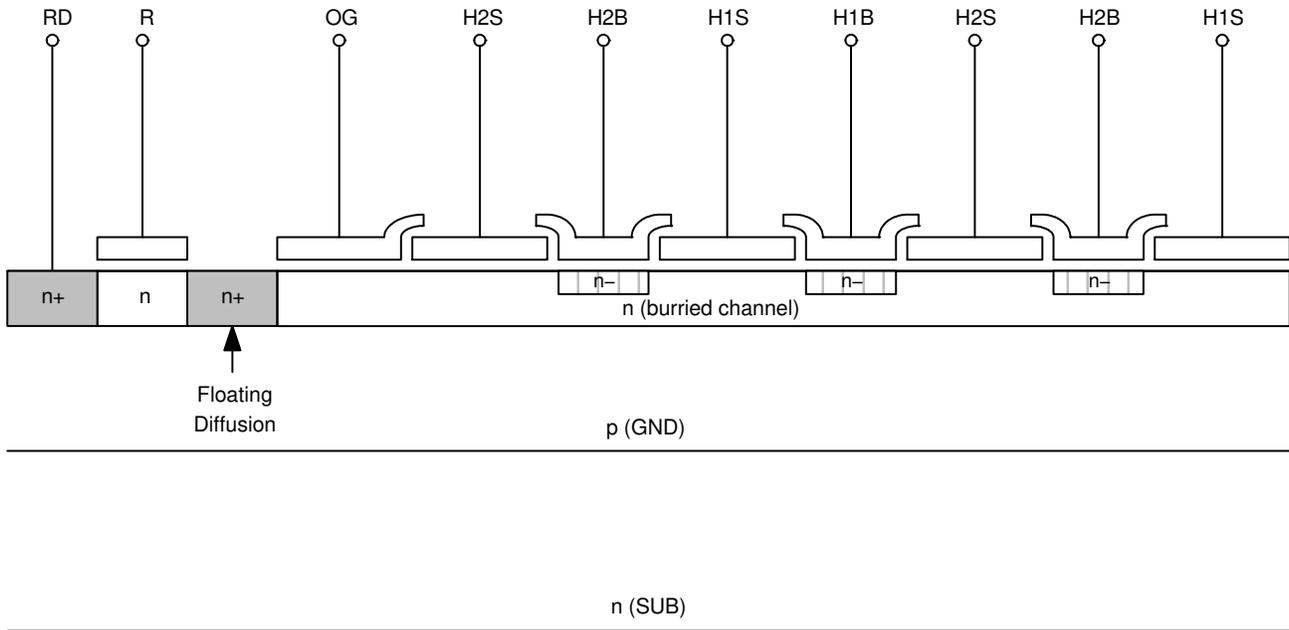
Figure 5. Horizontal Register to Floating Diffusion Architecture
