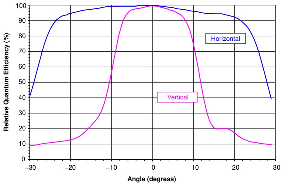
Figure 13. Monochrome with Microlens Angular Quantum Efficiency
