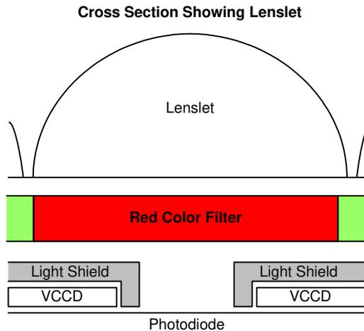
Figure 3. Pixel Architecture
