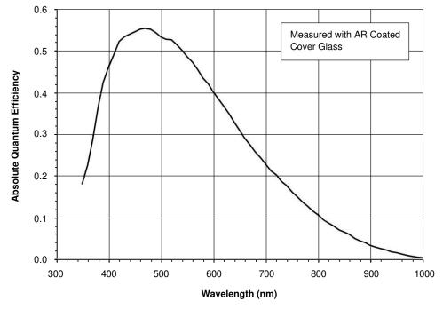
Figure 10. Monochrome with Microlens Quantum Efficiency
