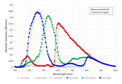
Figure 12. Color Quantum Efficiency
