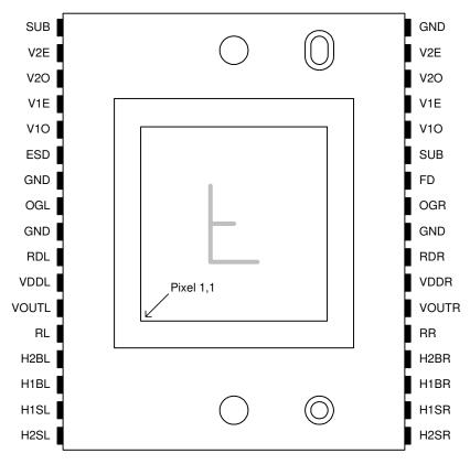
Figure 9. Package Pin Description- Top View
