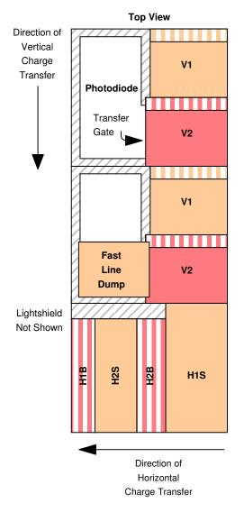
Figure 4. Vertical to Horizontal Transfer Architecture
