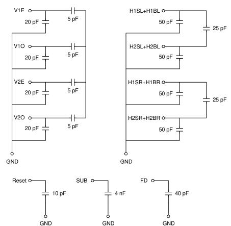
Figure 19. Clock Line Capacitances
