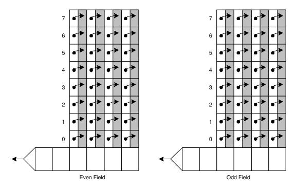
Figure 22. Summed Interlaced Scan Operation
