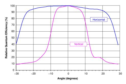
Figure 13. Monochrome with Microlens Angular Quantum Efficiency
