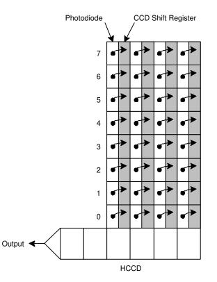
Figure 20. Progressive Scan Operation
