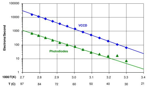
Figure 14. Dark Current vs. Temperature
