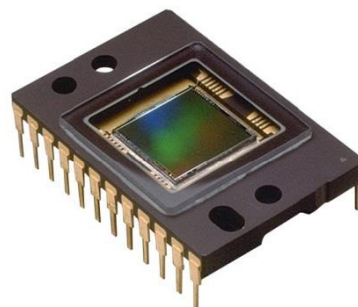
Figure 1. KAI-1010 Interline CCD Image Sensor
