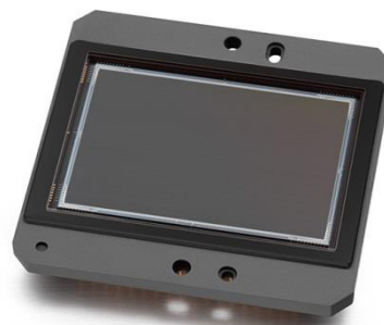
Figure 1. KAI-16070 CCD Image Sensor
