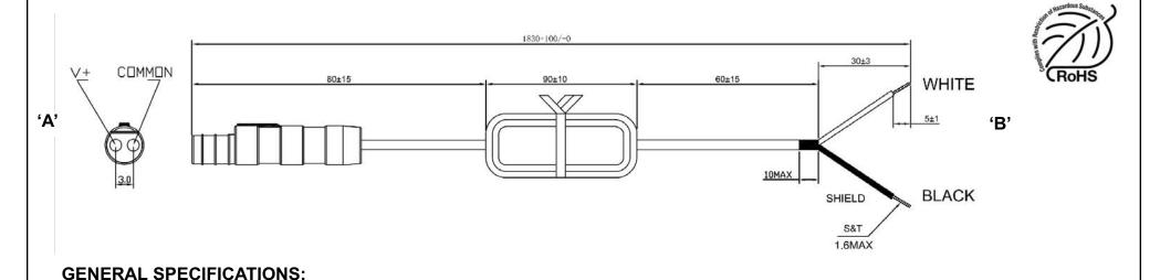
CABLE TYPE / SIZE: 1C+SHIELD, 20 AWG, FEP, PTFE, PVC, TFE, NEOPENE, POLYMIDE OR MARKED VW-1, 80°C,300V
