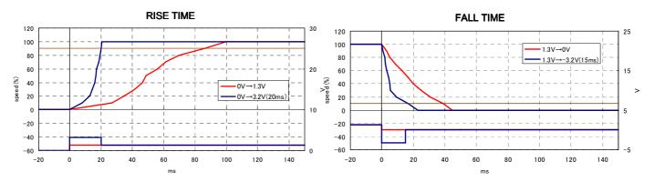
1.To reduce rise time, motor can be applied at 3.2V(20msec). 2.To reduce fall time, motor can be applied at-3.2V(15msec). \*please do not applied at 3.2V more than 30msec. \*please do not applied at -3.2V more than 30msec.
