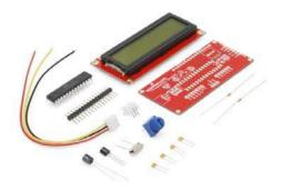
Description: This new revision includes a JST cable and also fixes the TX/RX swap from the last revision. Now you can use an FTDI correctly. We are also including a 16-pin header instead of a 40-pin header (only 16 pins are necessary).
