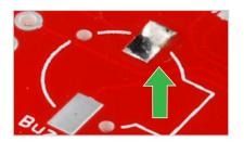
8 Using your tweezers, position the buzzer slightly away from the pad.
