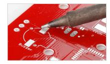
Pre-tin the start-pad by feeding solder into the joint.
