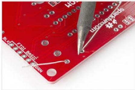
Feed solder into the joint.
