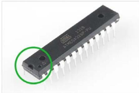
Now locate the position on the PCB. Again, notice a similar notch symbol in the PCB white ink:
