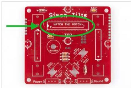
Taking care to align the notch properly, place the ATmega328 into the PCB. While soldering the first leg (it can be any leg you choose), make sure to keep the component flush with the PCB.
