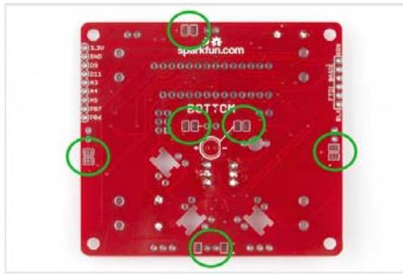
Each jumper has a small trace connecting the middle pad to the default polarity setting. The small trace is sometimes difficult to see, but it is a thin stripe of metal that should show up as a lighter color red. Using a hobby knife (aka x-acto knife), cut the default traces:
