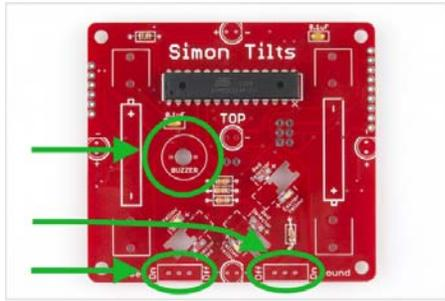
Place your components in the PCB. Flip it over and solder into place. When you are done, you're PCB should look like this:
