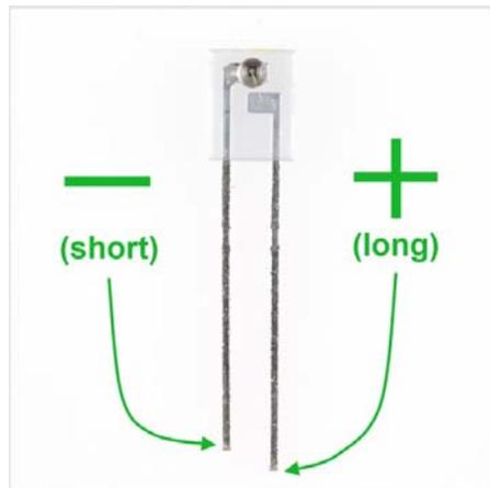
Locate the positions on the board. Notice that there are “Yellow Emitter” and “Red Detector” labels printed on the PCB. Also note that there are “-” and “+” marks for each leg. Be careful here to ensure correct placement and polarity.
