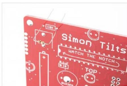
Push the resistor in so it is nearly flush with the board.
