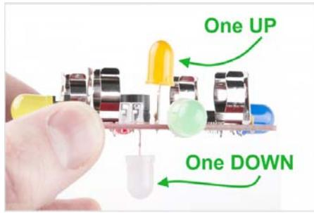
If you soldered in an LED backwards by mistake, have no fear. Visit the [Troubleshooting LEDs](#) section to find out how to easily correct it.
