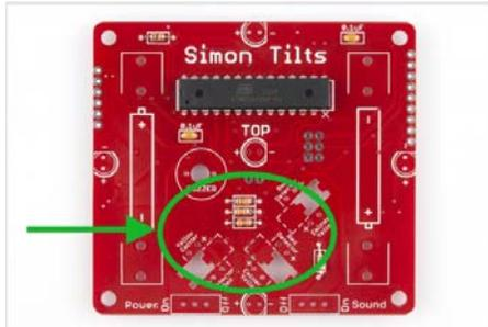
When soldering these into place, make sure they are positioned straight up (vertically). Check that your legs are forming a 90 degree angle with the PCB like so:
