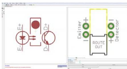
The package includes the correct positioning of the emitter, detector and dimension route out area to mate with the tilt arm part. An important thing to note is that when choosing a pull-up resistor for the detector line, we found that 330 ohms was the best value. This value is used in the kit. We first tried using the internal pullups on the ATmega328, but the voltage swing from the detector was very minimal which made it hard to get accurate readings.
