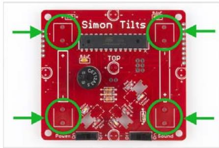
Note, these parts must be soldered in so the back sides are facing out. If placed incorrectly, the batteries will not fit. Ensure they are flush and that the back sides are facing out:
