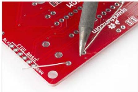
Feed solder into the joint.
