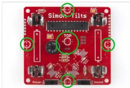
*Note: There are two LED positions in the middle of the PCB.*
