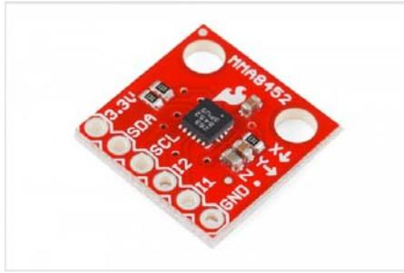
There was one problem with using a breakout board: the sensor itself is not a PTH part. Although we could include a footprint on the PCB to mate with the accelerometer's pinout, we were hesitant to use this approach. Adding one more "black box" to the project can increase the barrier to understanding a technology for a newbie.
