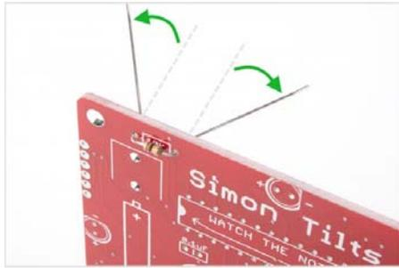
Flip the board over. Hold the soldering iron's "Sweet Spot" so it touches both the leg and the metal ring. Hold for 2 seconds.
