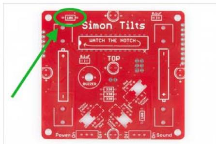
Insert the resistor into the PCB. Note, this component is not polarized and so it does not matter which leg goes into each hole. Some components on this kit are polarized, and we will take extra care when we get to them to ensure they are plugged in properly. To learn more about what it means to be polarized, please check out this tutorial: [Polarity](#)
