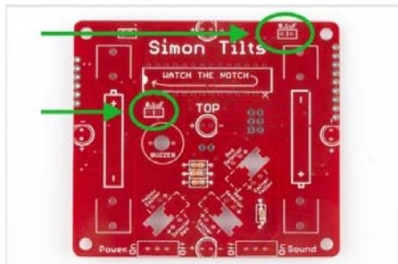
Ensure that they are flush with the surface of the PCB and standing upright. Solder them into place and clip access lead length. When you're done soldering these into place, your board should look like this:
