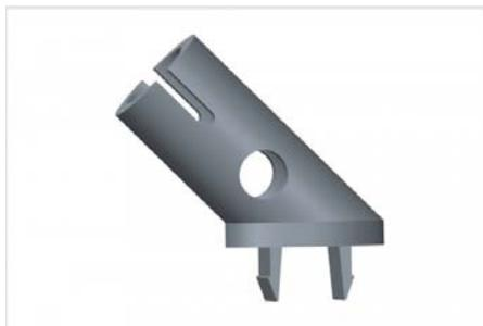
It uses an IR emitter and detector in order to know the position of the BB ball inside the cylinder. The IR emitter and detector are positioned so that the IR beam "shoots" through the hole in the bottom of the cylinder. When the BB is resting at the bottom of the cylinder, then it is blocking the IR beam. When the BB is resting at the upper end of the tilt arm, then the "look-through" hole is unobstructed, and the IR detector can sense the emitter.
