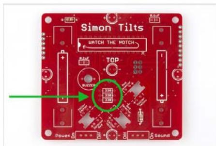
Using the same methods as before, solder into place and trim the extra lead length.
