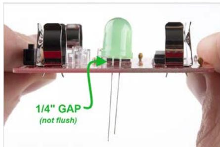
This will enable you to bend the LEDs outward like so:
