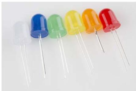
LEDs are polarized. This means there are "-" and "+" legs. Similar to the IR emitter and detectors, the LEDs have difference length legs to show polarity:
