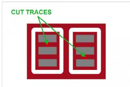
Using your soldering iron, close a jumper between the middle pad and the other outside pad:
