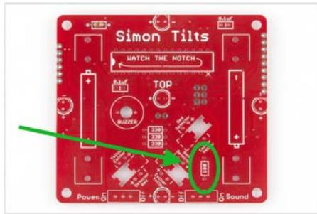
Using the same methods you learned with your first component (the 10K $\Omega$  resistor), solder into place, and trim the extra lead length.
