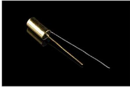
Each of these has a little metal ball inside that closes or opens a switch between the two leads. In this way of using a falling ball within a cylinder, it is very similar to our final Tilt Arm approach. The only difference is that the standard tilt sensor was not reliable enough for our application. We were getting very inconsistent readings from each sensor. Plus, the legs of those tilt sensors are pretty thin wire, and so after a little fumbling around, they would bend out of position.
