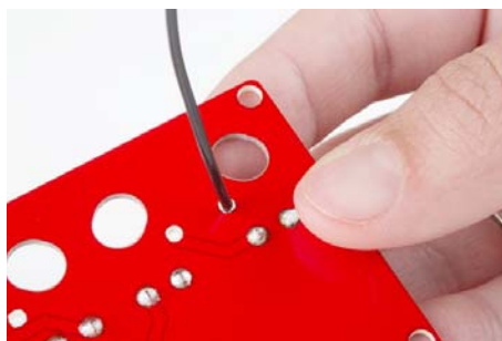
Prepped wire inserted into bottom of the board
