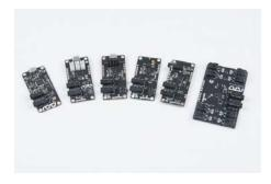
Spectacle launched with six modules: the Director Board, an Audio Output Board, a Motor Control Board, a Lighting Control Board, an Inertia Sensing Board, and a Button Input Board. Every Spectacle project consists of at least two boards: one Director Board and at least one of the output-type modules.
